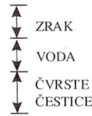
Totalna poroznost  $n = \frac{\text{Volumen pora}}{\text{volumen uzorka}} 100 = \frac{V_v}{V} 100$
